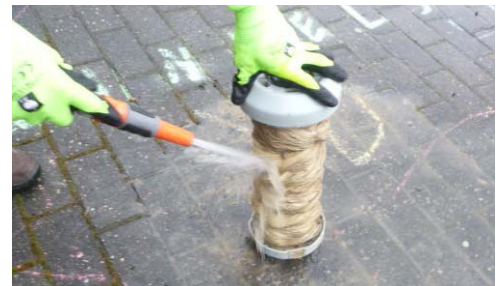
Fig. 7: Washing the membrane
