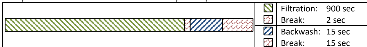
Figure 7: Filtration and backwash pump cycle
