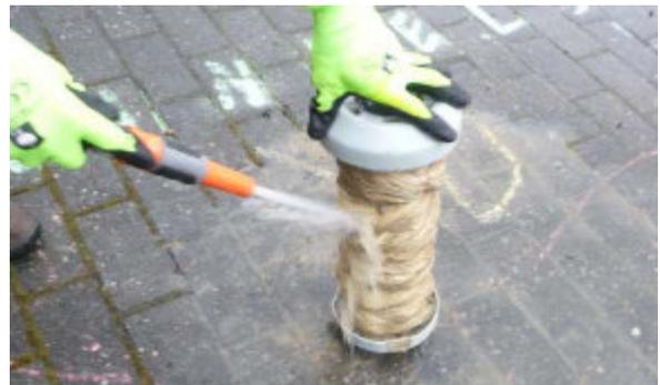
Rinsing the membrane fibre bundles
