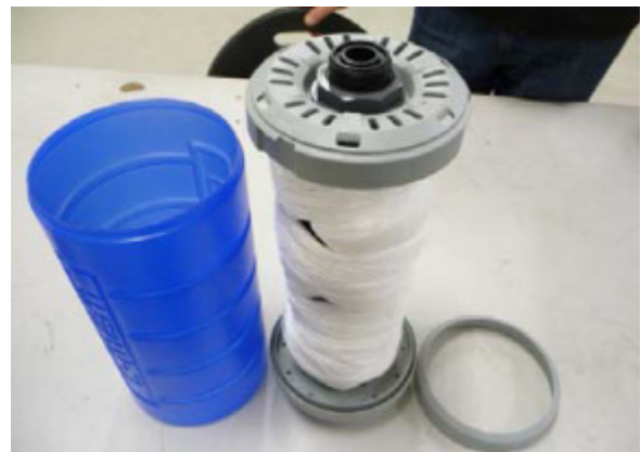
Blue outer jacket, membrane cartridge and outer ring
