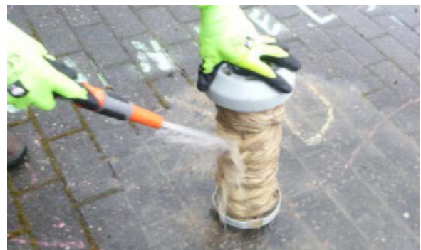
Rinsing the membrane fiber bundles
