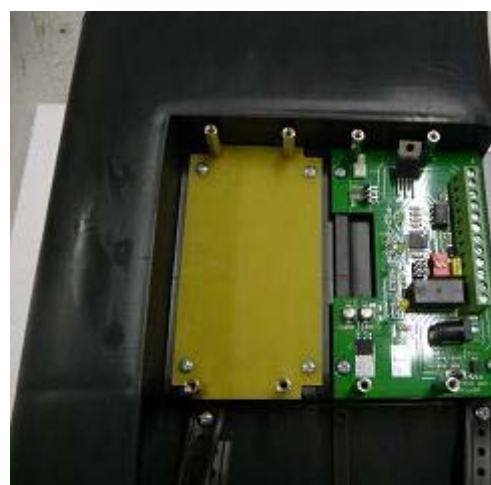
Remove left yellow front panel holder
